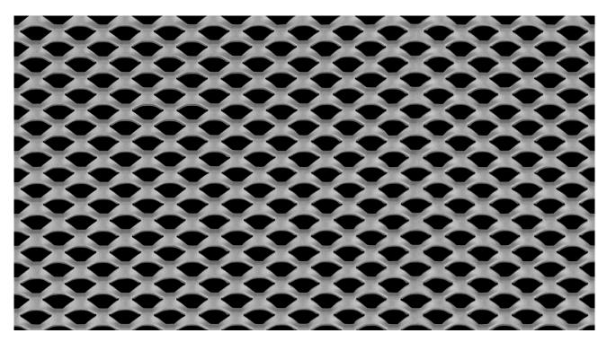
LW Pitch:12.70mmStrand Width:2.70mmSW Pitch:9.50mmThickness:0.90mmWeight:4.00 kg / m2Open Area:43%
